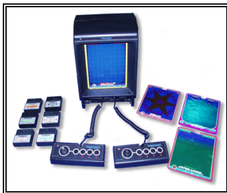
The Vectrex, a cartridge based vector console from GCE with colour provided by fitting a plastic overlay over the screen.
